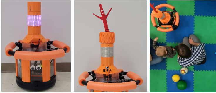
Fig. 1: Left: GoBot Bubbles, our custom robot with bubble, light, and sound stimulus hardware. Center: GoBot Dance, with air dancer hardware. Right: Partial overhead view of play space with robot, participant, and toys.
